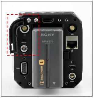
Before installing the E2 camera into the housing, screw the cable clamp on the camera as shown.
