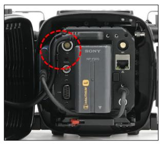
Connect the HDMI 2.0 cable through the camera's HDMI port as shown. The clamp is used to avoid over bending or twisting the cable and extend the cable's lifecycle.
